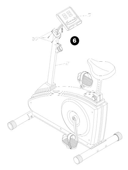
**6.** Connect the computer cable at the top of the console tube (2) to the console (5). Both computer cable connections have white ends. Feed the pulse wires from the console (5) down into the console tube (2) and out the rear hole in the handlebar area. Attach the console tube (2) to the console (5) with the screws (59) provided and already attached to back of the console (5).
